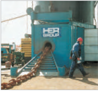
PE4004S pump and RD3006 cylinder used in a special press which repairs damaged chain links for the shipping industry.
