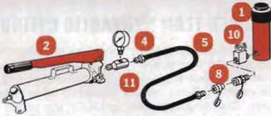
Basic single-acting system with a hand pump, gauge, hose and single-acting cylinder.
