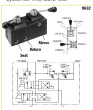
Pump mounted, 6-position detented 5way manual dual valve. Rated pressure to valve "A" is 10,000 psi and valve "B" is 6,000 psi. Case pressure is 500 psi max.
