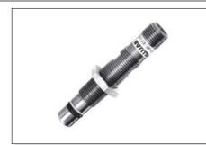
The inductive proximity sensors make it possible to detect metal objects; the operating principle is based on a high frequency oscillator which produces an electromagnetic field in the immediate vicinity of the sensor.
