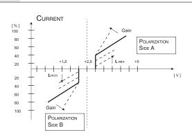
For being able to command a proportional valve double solenoid with a positive command voltage in income at contact 9 of REMD is necessary to connect the contact 10 of REMD a resistive load:
