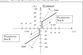
For being able to command a proportional valve double solenoid with a differential input command voltage in income at contact 9 of REMD is necessary not to connect the contact 10 of REMD.
