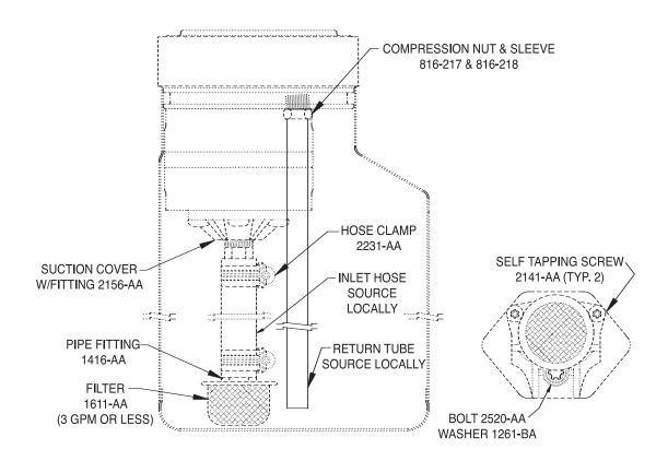
Parts may be assembled in either orientation depending on mounting of power unit.
